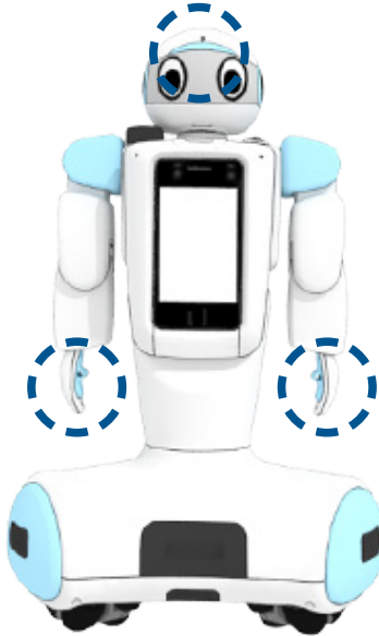
[Diagram 6–12] Touch sensor locations (both palms, head)
